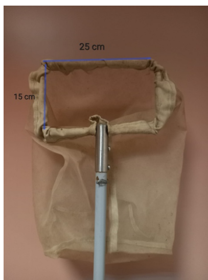
Figure 2.2. Macroinvertebrate sampling net with 25x15 cm with mesh size 500 \mu\text{m} , and 1.5 m long.
